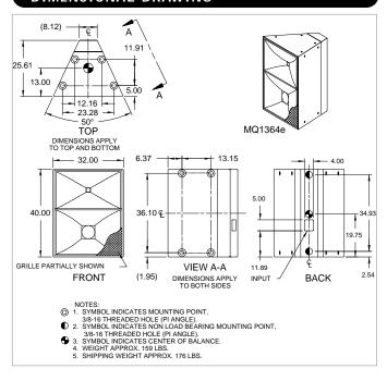
Manufacturing tolerances are +/- 0.13 and +/- 1 $^{\circ}$
